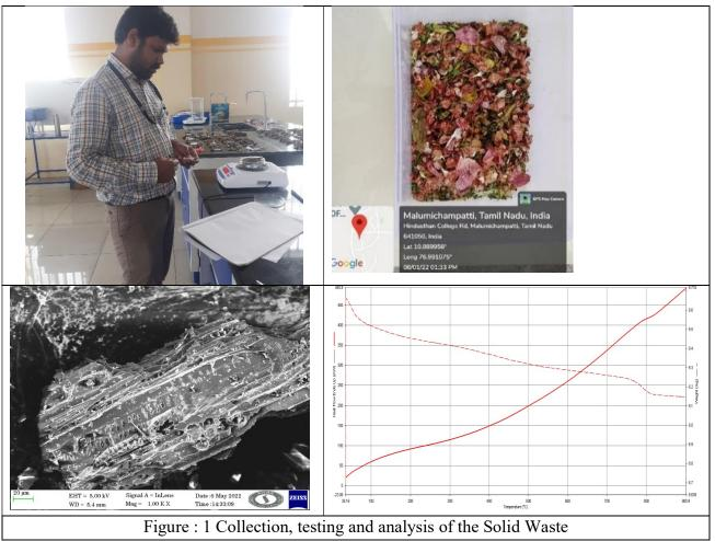
The thermal stability and fraction of volatile components of Sample are analyzed using TGA Analysis. From the TGA result, it is concluded that selected sample has good thermal stability. Kinetic behavior evidences that the biomass can be used for the energy recovery. The structure and the chemical Composition of selected sample was analyzed using SEM. The micro structure confirms that the sample is suitable for energy recovery purposes.
